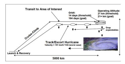
Figure 9. Hurricane tracking mission profile<sup>15</sup>
