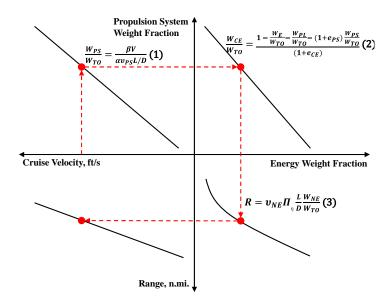
Figure 5. NAM ratio diagram plotting process<sup>14</sup>
