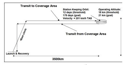
Figure 8. Communications relay mission profile<sup>15</sup>
