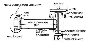
Figure 7. Open Brayton Cycle nuclear aircraft propulsion system schematic from 1977 Lockheed-Georgia report<sup>16</sup>
